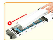
Insert the heat sink at 45° angle
